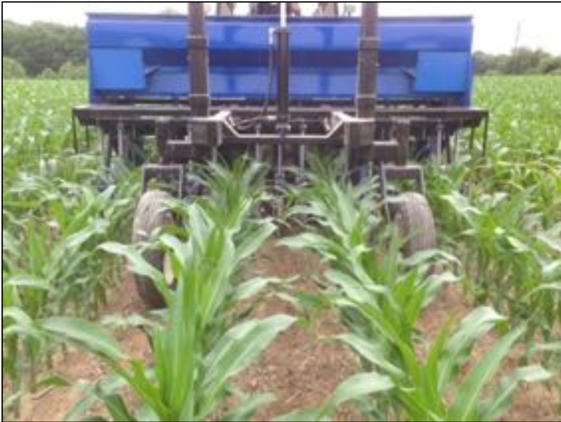
Interseeder used to seed a cover crop between rows of corn.
