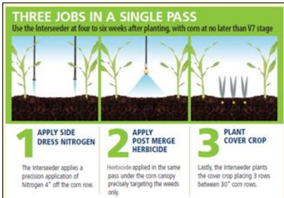
Interseeder used to seed a cover crop between rows of corn.
