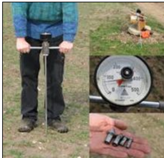
Soil penetrometer being pushed into the ground. A dial above the handles measures soil resistance. Lower inset shows the different tips that can be put on the business end of the probe.
