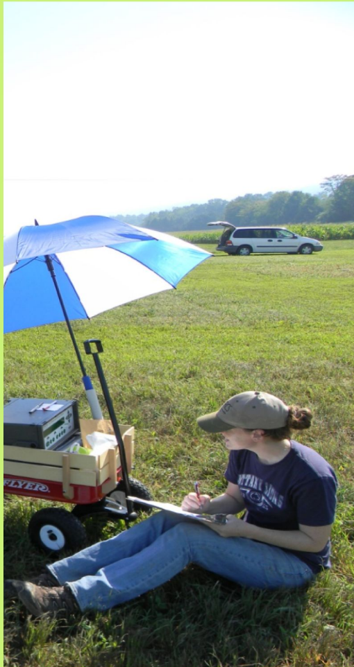
Measuring nitrous oxide and ammonia emissions with a Photoacoustic Analyzer
