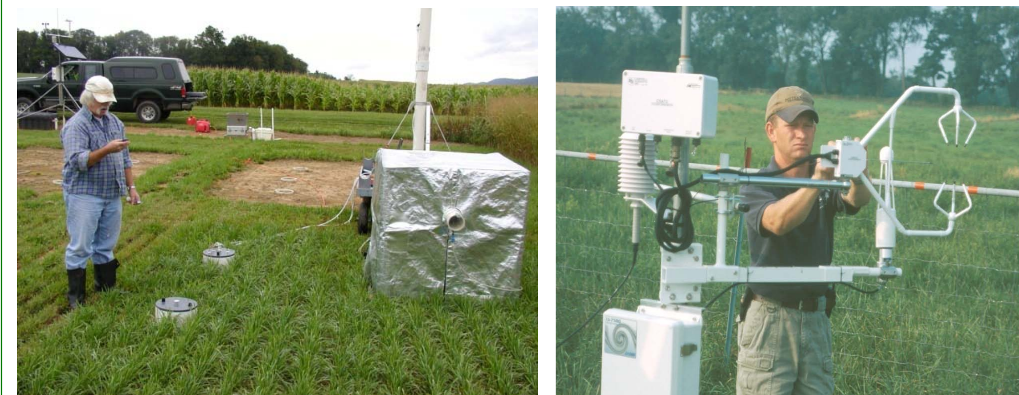
Measuring plant respiration (left) and carbon dioxide flux (right) from forage and pasture.
