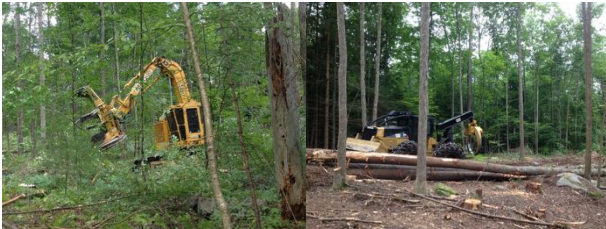
Feller-Buncher in operation
