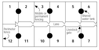
**Figure 6. Square or rectangular paddock layout.** This layout has a central lane with waterers shared between two paddocks. Paddocks are separated by mobile or permanent fencing.
