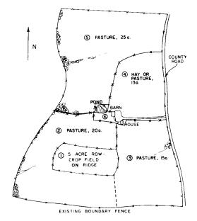
Figure 11. Subdivide the land into four paddocks using permanent (x-x) and temporary (--) fencing
